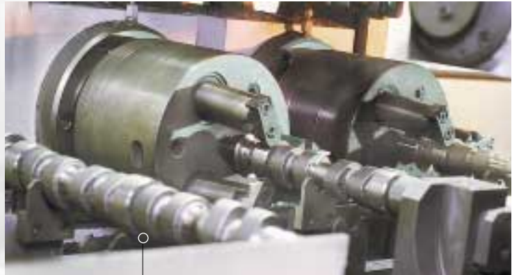
• Hermetically sealed chucks fitted in a milling and boring line. Photo: Courtesy, VW in Salzgitter
