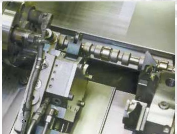
• Camshaft machining with steady rest. Photo: Courtesy, VW in Salzgitter
