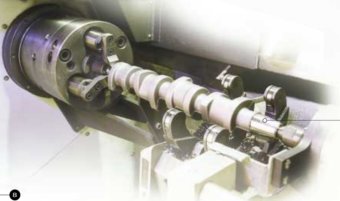
• Partially machined camshaft with steady rests. Photo: Courtesy, VW in Salzgitter
