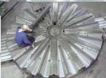
12 WAZK 4000 The largest 12 jaw power chuck in the world - 4000 mm dia.
