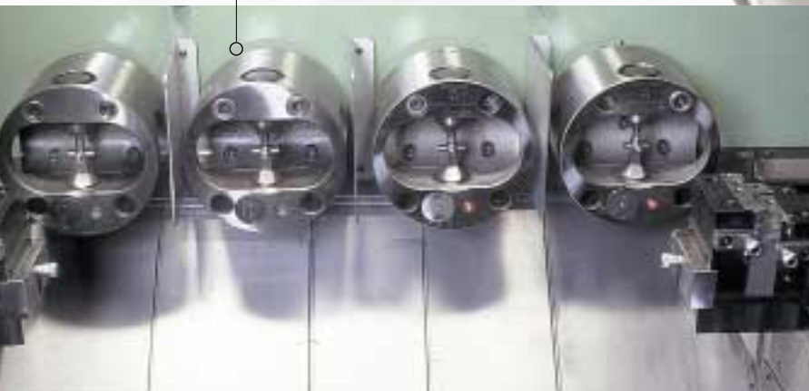
• Large batch production using hydraulic indexing chucks within a multi-spindle machining application.
