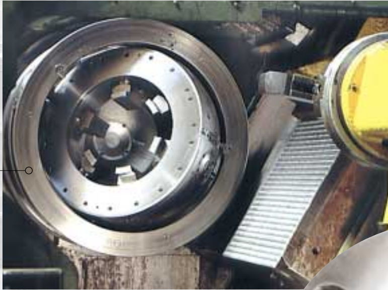
• Hydraulic indexing chuck for the complete machining of threaded sleeves.
