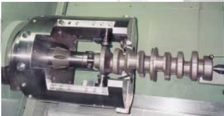
Special design for heavy vehicle crankshafts for secure workholding and accurate machining.
